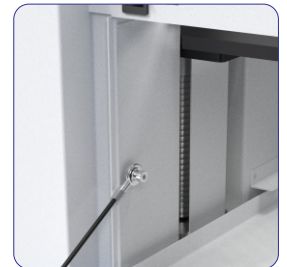
Z Axis work table 182mm max part height.
