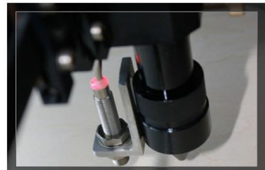
Auto focus Help the user to set the focus Easier. (based on motorized table).
