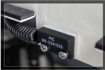
Open flap protection Laser will stop working if you open the front cover.
