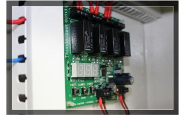
Smart Board Control the exhaust fan, air assist, and alarm lamp automatically, energy saving.
