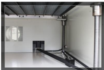
Motorized table Control the table up/down from LCD panel directly.
